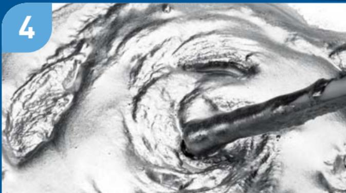
Once a homogeneous paste is achieved then the ink can be finished by adding the necessary resins and additives in portions with gentle mixing.
