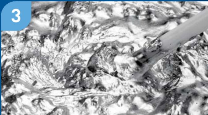
After a minimum of 30 minutes gently stir the mixture with low shear mixing, preferably using a paddle blade covering 65-70% of the vessel diameter, until a homogeneous paste is obtained.
