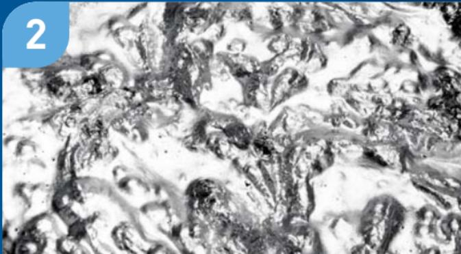
Add to the granules an equal weight of solvent and allow a minimum of 30 minutes soaking. As soon as the solvent is added the granules will visibly start to disperse as the solvent wets out each flake.
